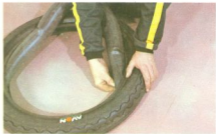
Tyre fitting: Inflate inner tube and insert in tyre
