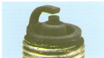
Black sooty deposits indicate an over-rich fuel/air mixture, or a malfunctioning ignition system. If no improvement is obtained, try one grade hotter plug
